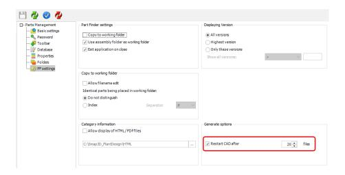
The reason for the development of this new option is a behavior of all 3D CAD systems we support when you call up the automatic creation/generation of 3D files from "outside" via the programming API of the 3D CAD systems.
