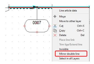
After clicking on this function, the representation of the secondary line (in relation to the main line) for the previously selected lines is mirrored according to the initial situation.
