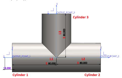
2. The 3D components require the user-defined parameters **Lmin** and **Lmax** with appropriate values for the allowed **minimum** and **maximum length** of the respective leg/orbital cylinder.
