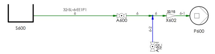
Some customers who have used the **Pipeline list** tool since its introduction in version 2023 have asked us over the past few months, to adjust the algorithm for the evaluation results. These requests applied to the cases of line-to-line branch situations in diagrams, in conjunction with the active **Exclude opposite flow** option.
