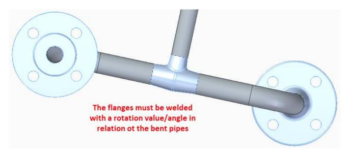
To better support our customers with this important manufacturing requirement during 3D pipeline planning, we have developed the new **Calculate component rotation** function for Smap3D Piping.
