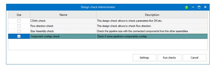
When running this design check, the coordinate systems (INPUT/OUTPUT) contained in the fittings are checked for overlap, not their solid model.
