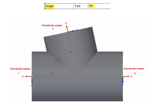
If all requirements are fulfilled, it is now possible to create very flexible and automatic individual pipelines with different tee branch angles without having to place the special tees manually at the branches.
