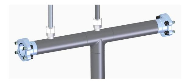
From the point of view of Smap3D Isometric and Isogen, the difference so far has been whether such a branch is placed on a pipe or a tee-piece fitting.
