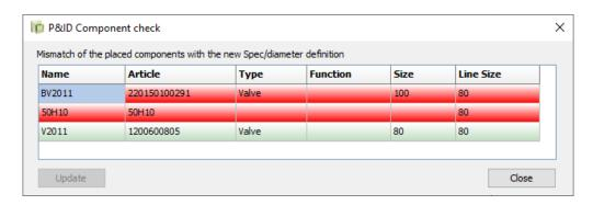
This process should be repeated for all components displayed in red if this is possible with the contents of the new pipe spec/diameter definition.
