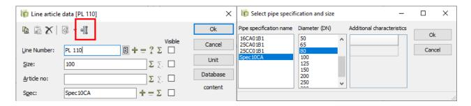
For all pipes/lines defined this way, users can use the **Place from specifications** function to place the appropriate components defined in the respective pipe specifications.
