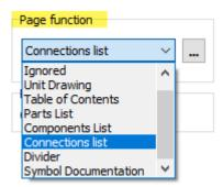
After inserting a user-specific template page into a project, it must be displayed as a **NET** page type.
