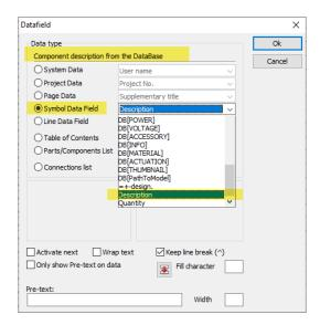
If this symbol data field **Description** is defined and used in a symbol, a user can manually enter a value for it if there is no article assignment from the database for this symbol.
