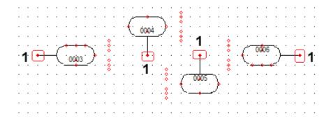
If all prerequisites are fulfilled, a connected PCE symbol can be moved in a diagram and the respective connection line dynamically adapts to the corresponding distance to the line.
