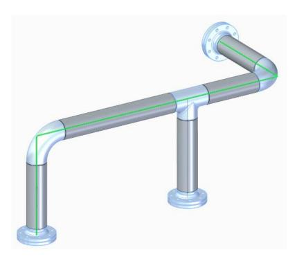
After clicking on **Split route**, a dialog appears. After selecting the component and the coordinate system at which the route should be split, the automatic operation is started with **OK**.
